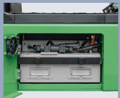
Lithium Iron Phosphate Battery Pack
