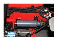
There's an energy accumulator applied in the braking system, which means when the engine is shut down,it can also provides more than 4 times emergency brake.
