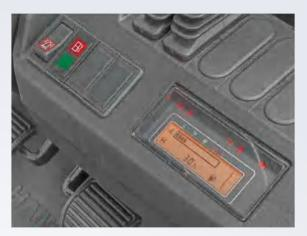
Newly developed LCD meters have more complete functions and more stable performance. Important information including running status of the entire truck and failure of the engine (electronically controlled engine) can be displayed completely, so that the operator can understand status of the truck in a visualized manner, for easy maintenance.
