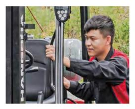
Large hand grip Large hand grip of optimized design enables easier access to the truck.
