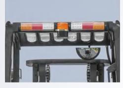
LED lights are applied for entire truck. It saves power and energy, with significantly increased performance and service life of lights.
