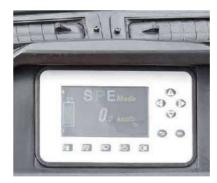
The large LED display screen has functions of electric quantity display, timing meter and failure self-diagnosis. Without the handheld unit, changing vehicle performance and overhaul can be completed via the instruments. The failure will be displayed both in code and text, which is more visual and easy for reading.
