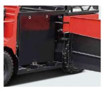
The battery can be replaced through being hoisted or laterally moved out, which provides convenience for use by the user.
