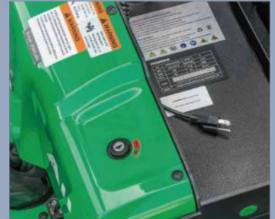
Features a built-in charger and a maintenance free battery.
