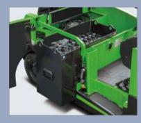
The Tow Tractor features a battery side roll out in order to replace the battery fast and easy.
