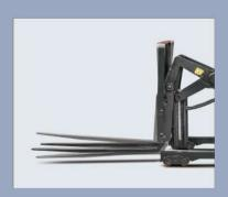
The forks' tilting function is easy fo loading and unloading pallets.
