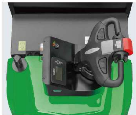
The tiller and instrument display can be moved sideways to allow for more room when changing the battery.
