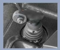
The intuitive, multifunction control handle is centrally positioned for easy access. The handle offers simultaneous control of the drive, lift, lower, and auxiliary hydraulic functions.
