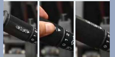
Three forward gears- Suspension hydraulic transmission with three forward gears, top speed reach 15.5mile/h
