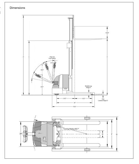
Note: Aisle dimensions listed above assume the bay width to be straddled OD plus 2" (1" on either side of straddle Ieg). Straddle OD is the load width plus 8". \*For metric conversion multiply inches by 25.4.
