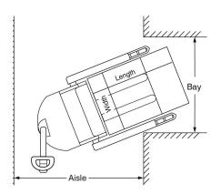
Note: Aisle dimensions listed above assume the minimum bay width to be straddle OD plus 5" (2.5" on each either side of straddle leg). Straddle OD is the load width plus 10". Truck performance may vary due to application requirements and changes in model design.
