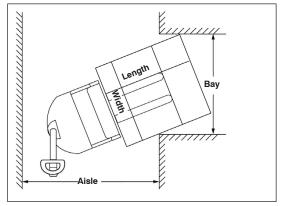
Note: Aisle dimensions listed above assume the larger dimension; load width or load length. For ease of use and add 6° to 12" for operator clearance to the appropriate specifications listed above. Truck performance may vary due to application requirements' and changes in model design.
