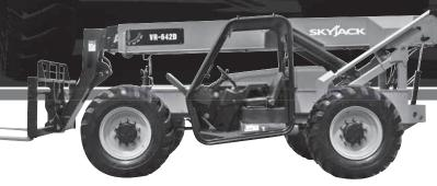
Skyjack's VR642D offers higher reach, greater capacity, and improved visibility, all to boost your jobsite productivity. With a maximum capacity of 6,700 lbs. (3,039 kg) and a lift height of 42' (12.80 m) the VR642D offers the same industry leading rugged, robust, and reliable design features that Skyjack is famous for. Ideal for residential construction trades, the VR642D features a boom design and machine construction that offers unsurpassed jobsite capabilities.
