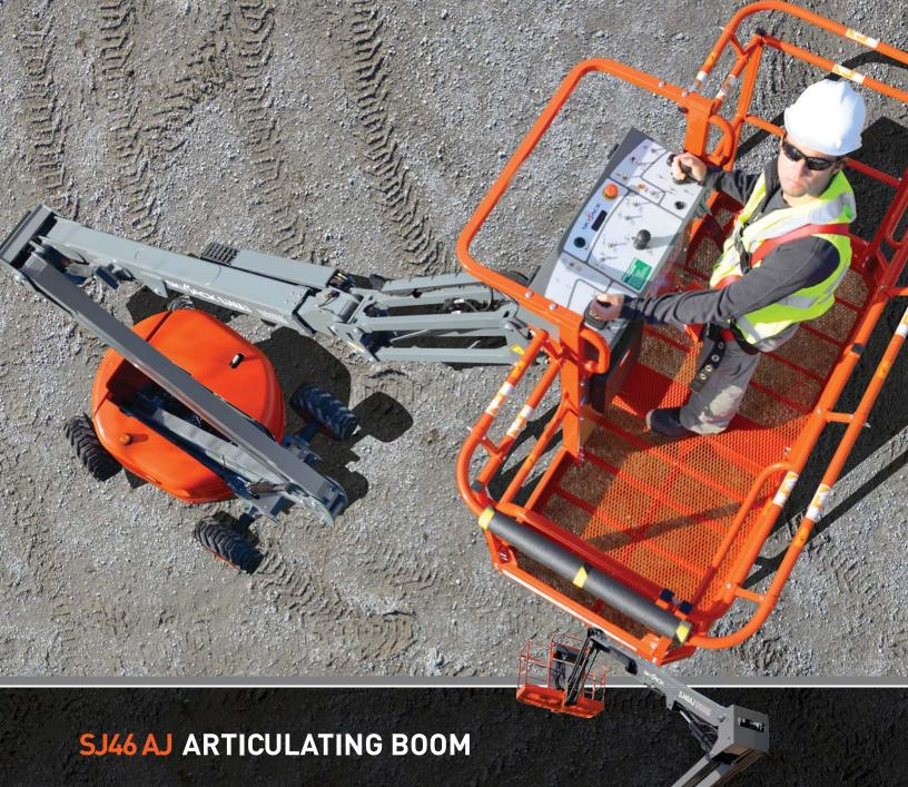
The SJ46AJ boasts an industry leading, standard equipped, 360 degree continuous turret rotation. Zero tail swing compliments the turret design allowing for flexible operation in tight locations. Superior positive traction and terrainability is provided by the axle based 4WD used in many of Skyjack's product designs, which accounts for a proven low maintenance, rugged and reliable drive train.
