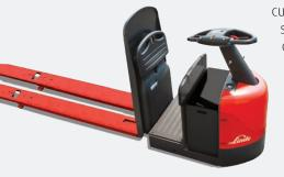
cushioned operator platform, soft-touch accelerator controls as well as adjustable steering columns. Standard knee cushions and lean-on seat round out an ergonomic package designed to maximize operator comfort. The ETR Series tractor series is designed to operate in indoor environments, towing trailers requiring up to 750 pounds maximum drawbar pull.
