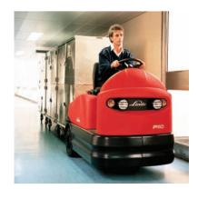
A rugged steel chassis is combined with a one piece, heavy duty polyethylene top moulding to protect the operator within a spacious compartment, with all controls ergonomically grouped for easy, fatigue free driving and manoeuvring.
