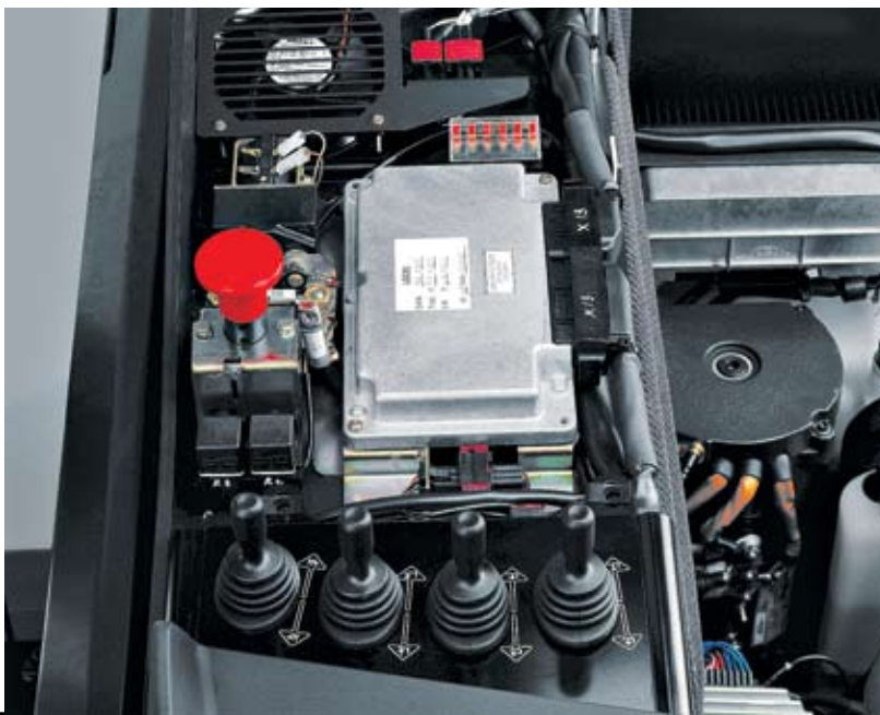
Efficient conversion of energy to motion. Linde Digital Control with CAN bus connection.
