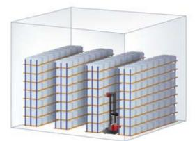
In a conventional warehouse, the aisle width required is over 2.7 m.
