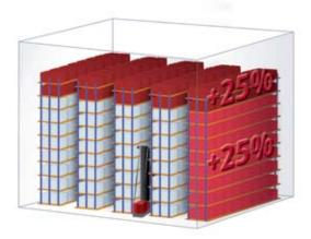
Unlike a conventional warehouse, the aisles in a VNA warehouse are around 1.7 m wide gaining +25% of storage. VNA racking can also be substantially higher, enabling around 50% more storage compared to a conventional racking system.
