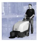
Walk-behind scrubbers are well suited to smaller facilities with a need for scrubbing and light debris pickup.
