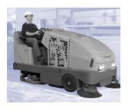
For facilities that require both sweeping and scrubbing, sweeper-scrubbers combine two cleaning functions into one machine.
