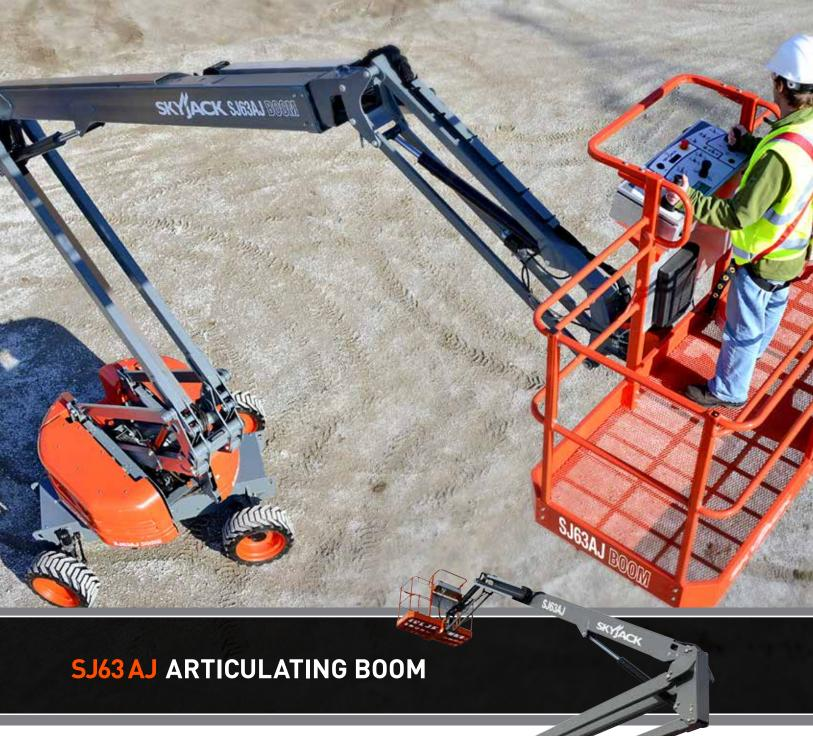
Combining a working height of 69'7" (21.2 m), a horizontal reach of 40' (12.2 m), and an up and over clearance of 27'6" (8.4 m), Skyjack's SJ63 AJ is designed for versatility. Superior positive traction and terrainability is provided by the axle based 4WD used in many of Skyjack's product designs, which accounts for a proven low maintenance, rugged and reliable drive train. 360 degree turret rotation and zero tail swing allow for flexible operation in tight locations.
